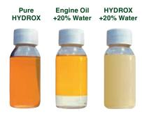
HYDROX and NEOX lubricants dramatically reduce wear to sterntube bearings in the event of seawater ingress.
